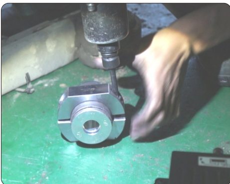
Installation of the lug pin.
